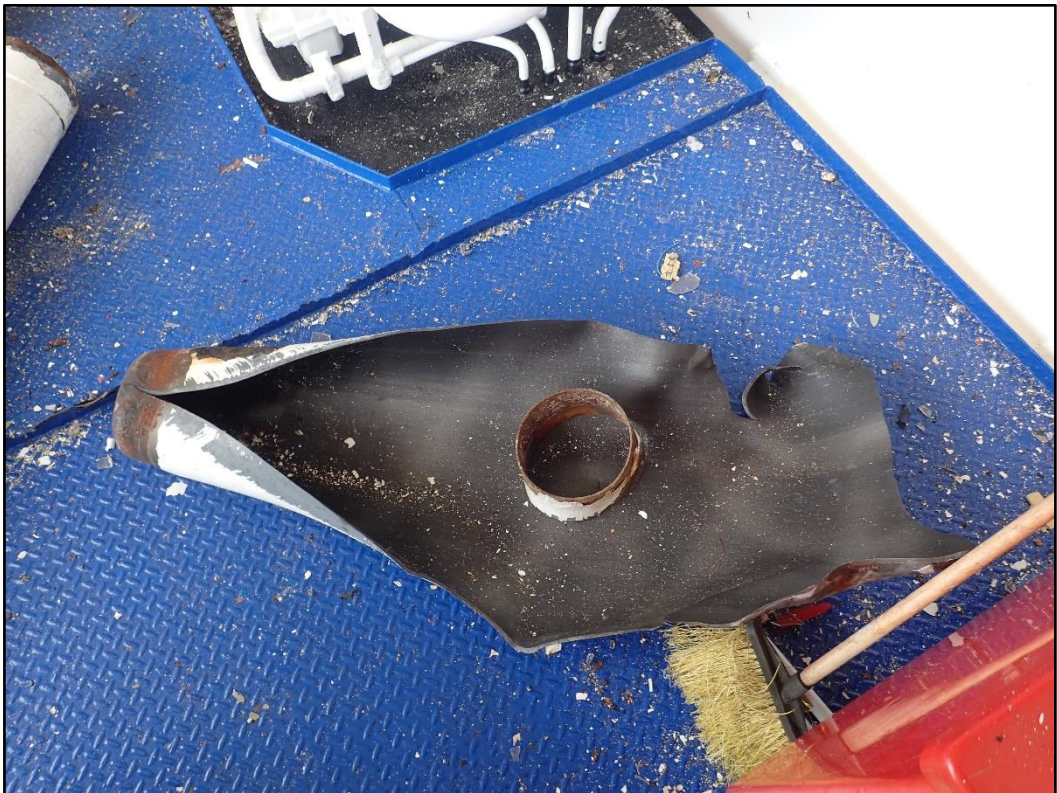
Figure 5 Failed nitrogen cylinder
