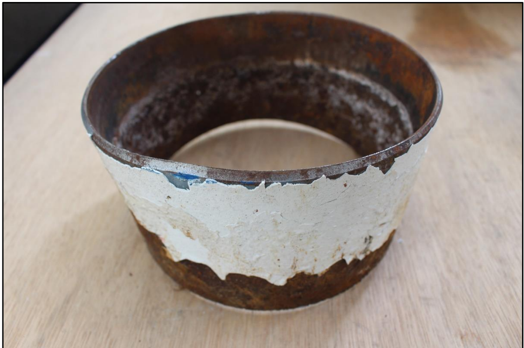
Figure 12 Foot from failed cylinder
