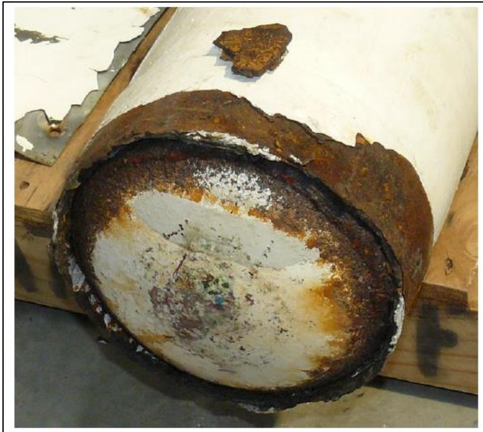
Figure 13 Extreme corrosion at the base of the randomly selected cylinder under the foot ring
