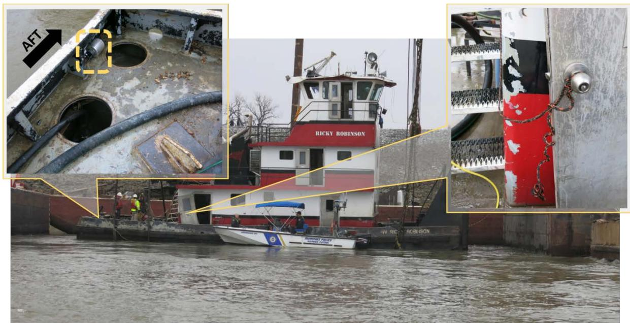
***Ricky Robinson* post-salvage. Two inset photos show, at left, both aft voids missing hatch covers, with a yellow square highlighting where submersible pump was found, and, at right, open starboard engine room door tied off to stairs.**
