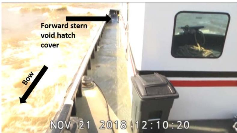
**Screenshots from Wepfer Marine video of *Ricky Robinson* in a lightboat condition while heading into two different current speeds. In each instance, when vessel speed increases, the amount of water coming over bow increases.**
