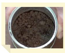
PASS Free particles Not flattened out No free water on surface
