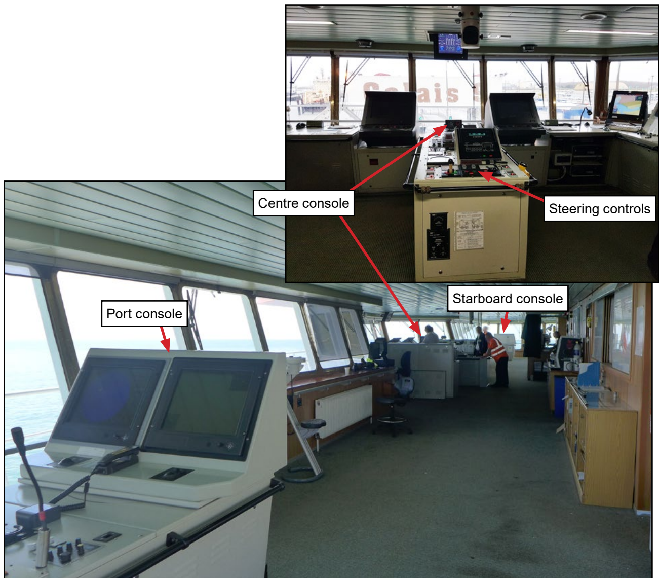
Figure 9: Fully enclosed bridge arrangement
