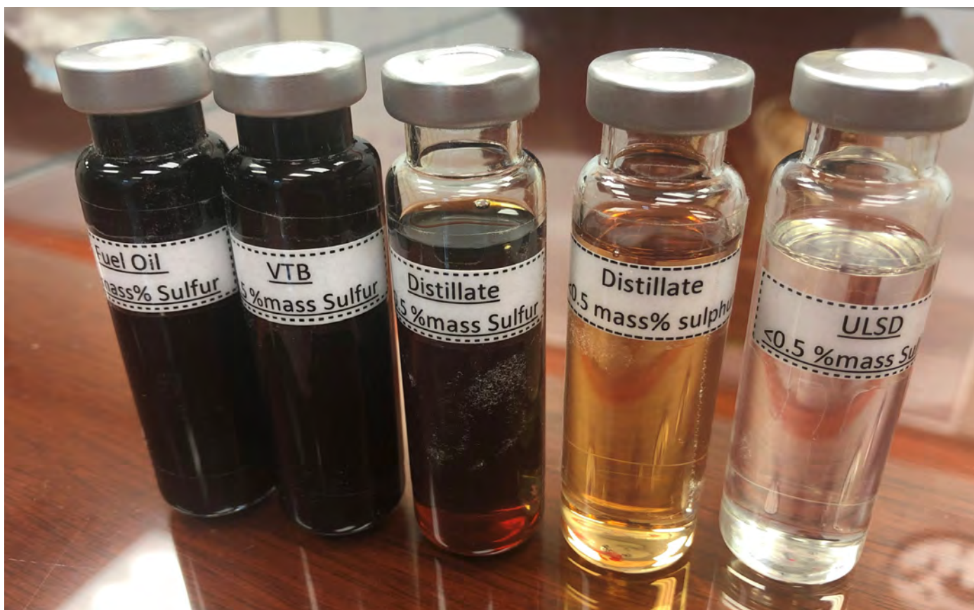
Figure 4.1 | Range of <0.5% sulfur samples including marine fuel oil, vacuum tower bottom (VTB), two distillates and ultra-low sulfur distillate.
