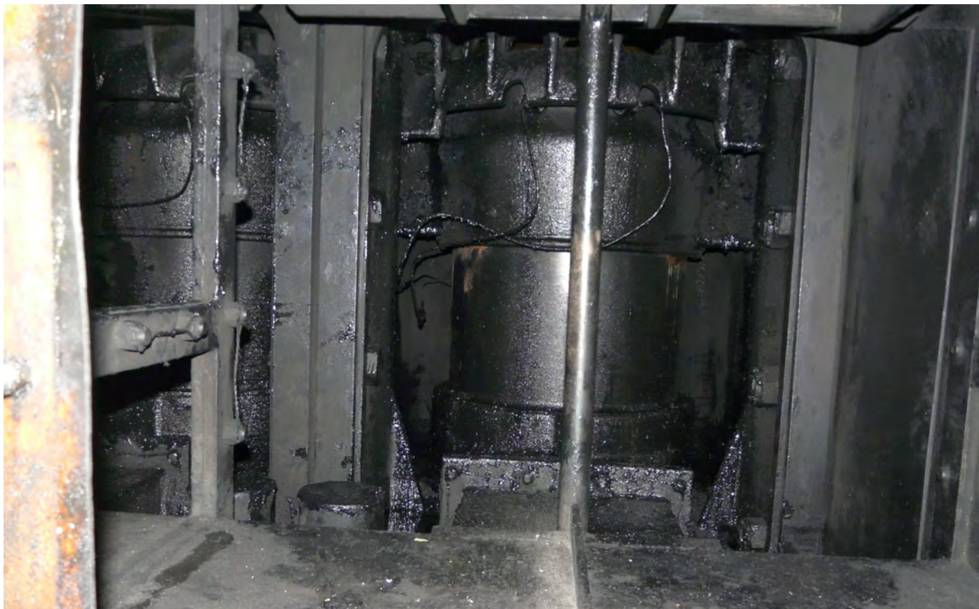
Figure 2.4 | Scavenge space charred after fire
