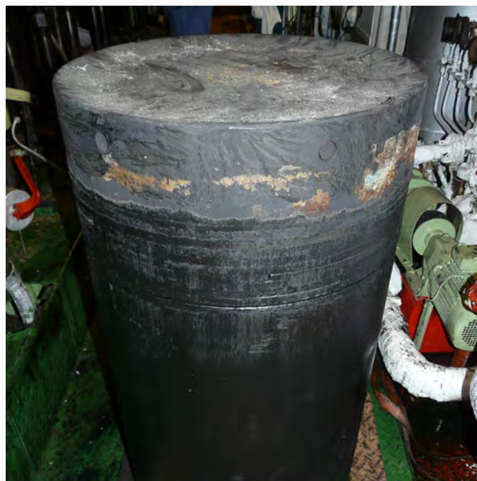
Figure 2.6 | Piston crown & rings heavily carbonized
