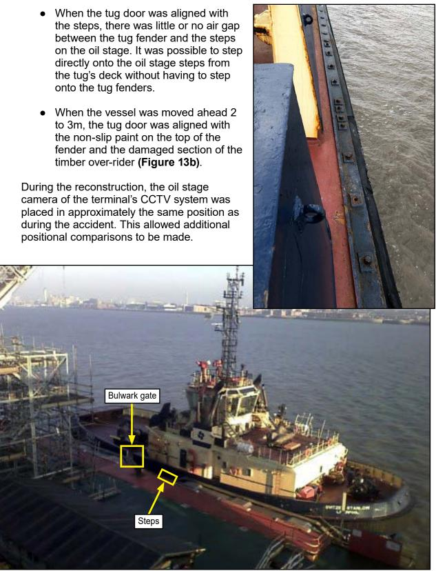
Figure 12: Svitzer Stanlow (inset: Svitzer Stanlow's 'rubber iron' outside the bulwark)
