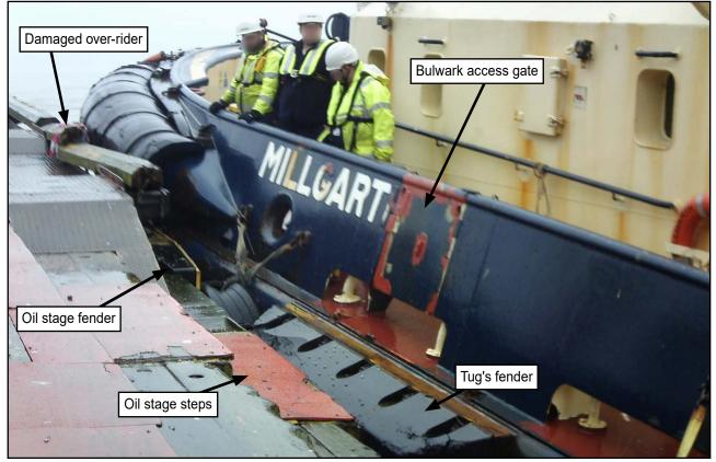
**Figure 3:** Oil stage steps and *Millgarth*'s bulwark access gate (photograph taken during post-accident reconstruction)
