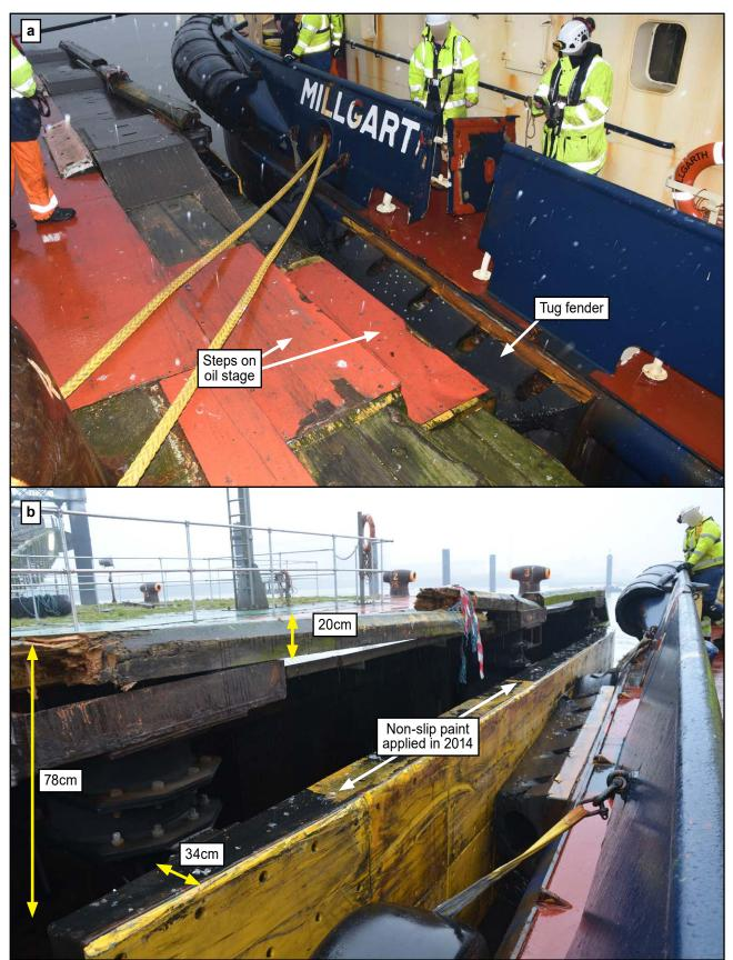
**Figure 13:** Reconstruction (**a:** tug gate aligned with the steps, **b:** approximate location of *Millgarth* when chief engineer attempted to board)
