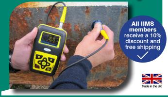
Tritex NDT specialize only in the manufacture and supply of Multiple Echo Ultrasonic Metal Thickness Gauges, used for verifying corrosion levels and measuring metal thickness from one side only, without removing any protective coatings.
