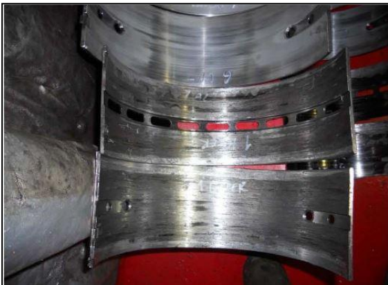
Figure 1: Big end bearing of cylinder no. 1 (scouring)
