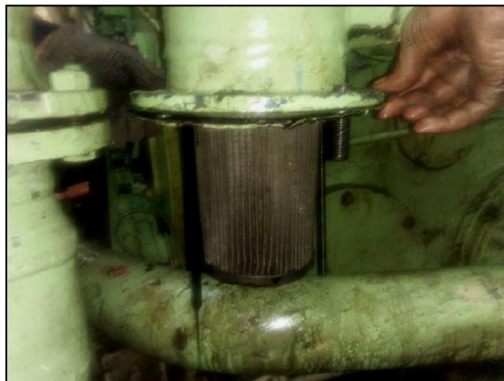
Figure 12: Extraction of the filter cartridge
