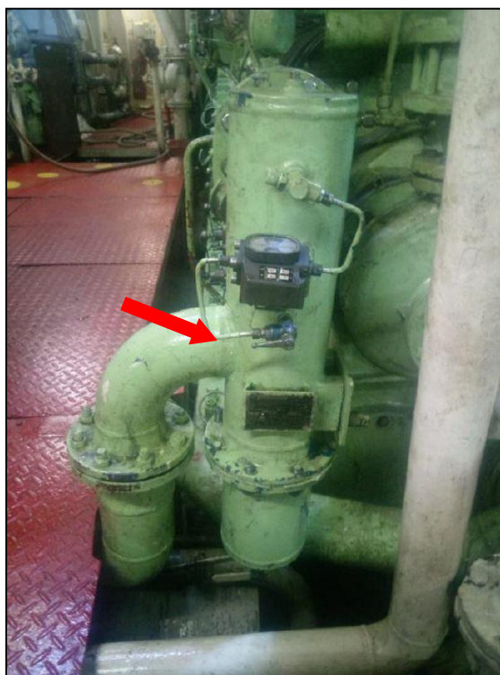
Figure 13: Position where the upper end of the filter cartridge was pressed
