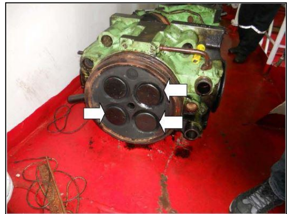
Figure 4: Cylinder head no. 1 (bent valves)
