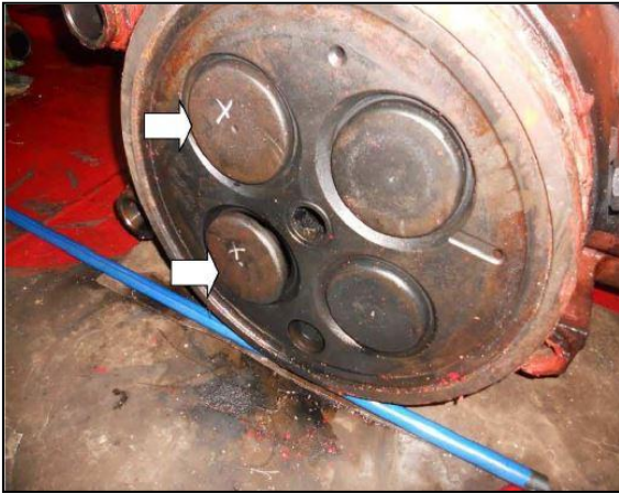
Figure 6: Cylinder head no. 6 (bent valves)
