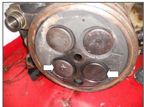
Figure 5: Cylinder head no. 3 (bent valves)
