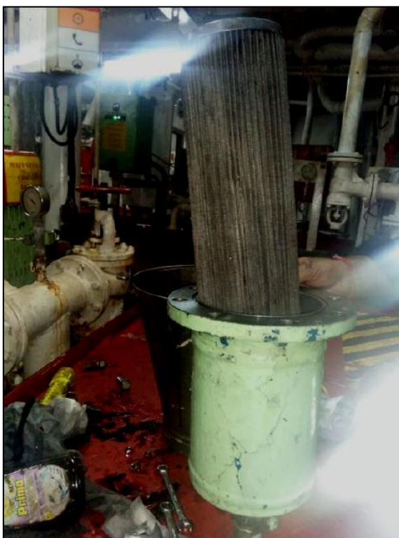
Figure 14: Simulation showing the angle at which the filter cartridge was found mounted
