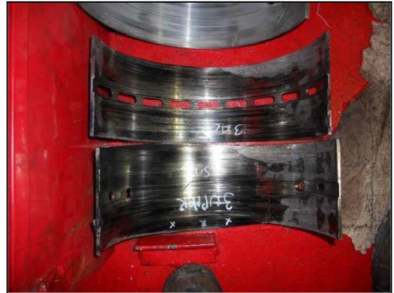
Figure 3: Big end bearing of cylinder no. 3 (scouring)
