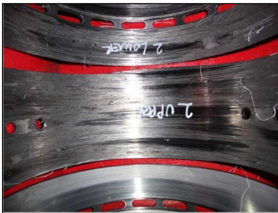
Figure 2: Big end bearing of cylinder no. 2 (scouring)
