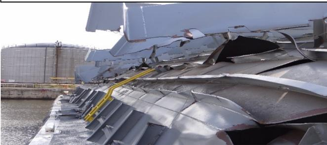
**Bulkhead between the #1 from the #2 cargo tank, folded/breached**
