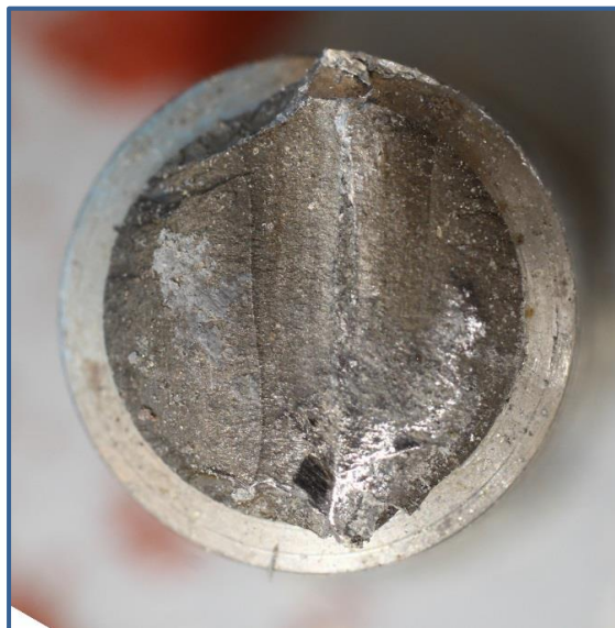
Figure 13: Fatigue fracture surface of a stud-bolt from the Discovery 2
