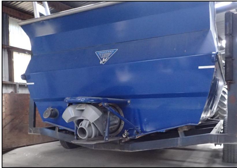
Figure 7: The jet unit installed on the Discovery 2 prior to its removal after the accident
