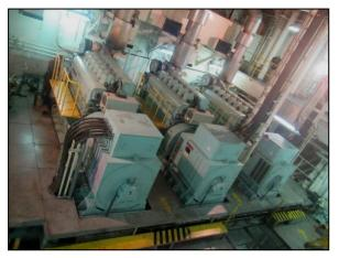
Figure 1: Auxiliary engines on board Leopold LD
