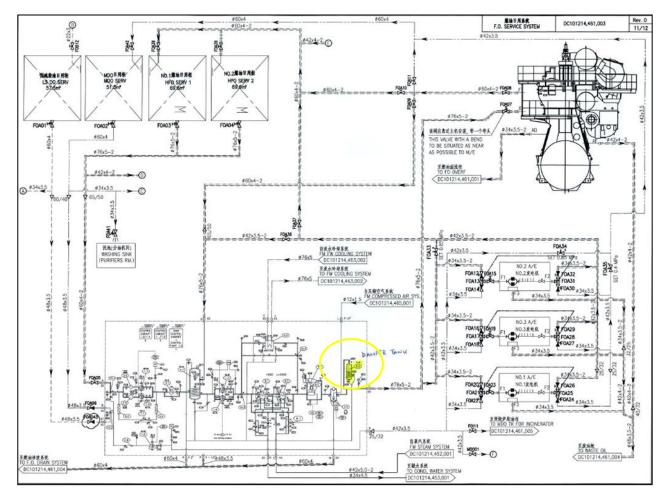
Figure 7: Fuel oil service system, showing the damper tank in yellow
