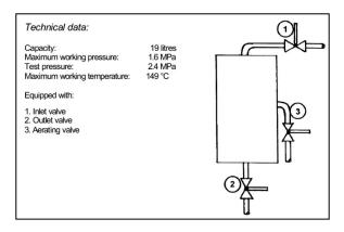
Figure 8: Side elevation of the compensation damping tank
