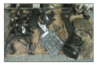
Figure 3: Damaged components on A/E no. 2
