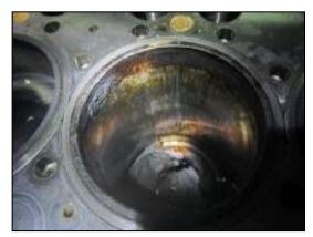
Figure 5: Damaged cylinder liner
