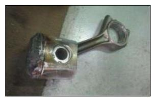
Figure 4: Damaged piston and connecting rod of the emergency generator
