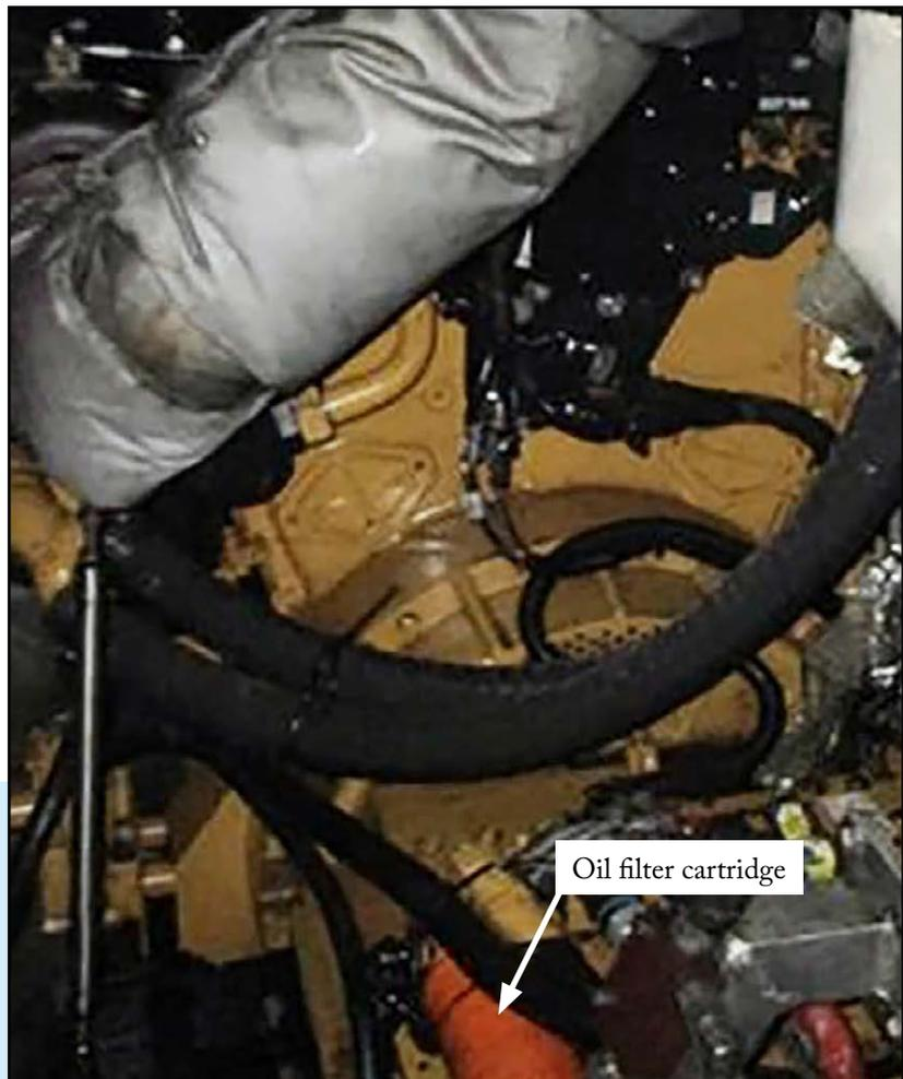
Figure: Clutch hydraulic oil filter cartridge
