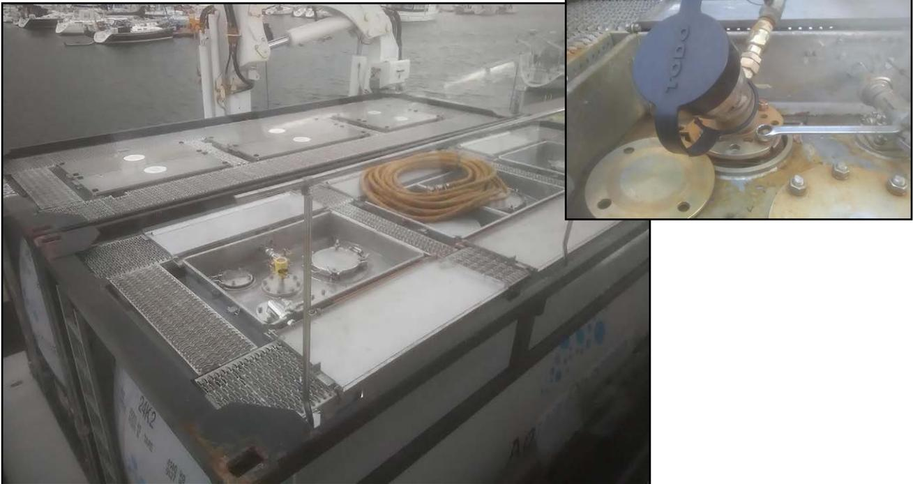
Figure: The hydrogen peroxide tanks as seen from the wheelhouse (inset: the valve being removed)
