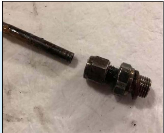
Figure: The failed compression fitting (olive not shown)
