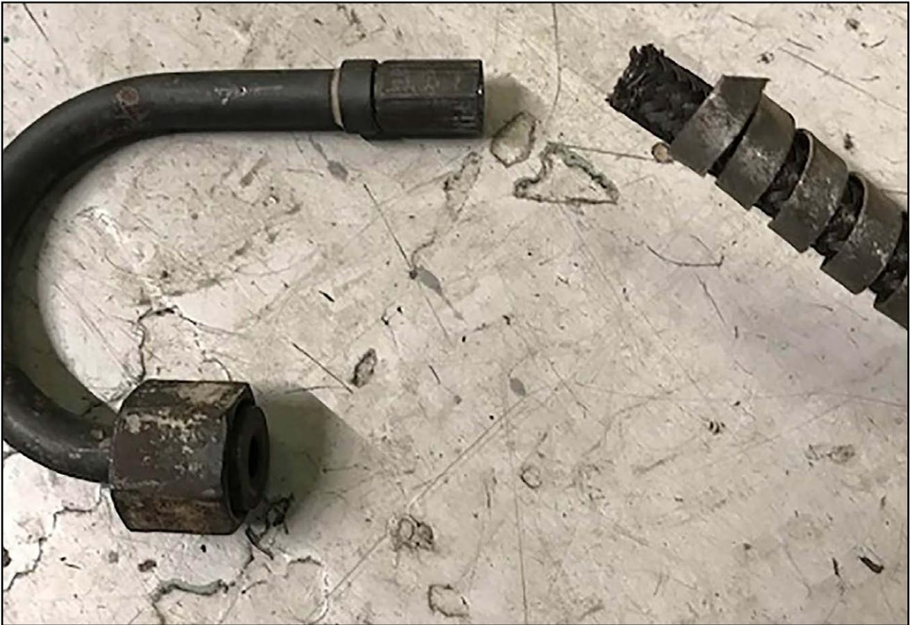
Figure 1: The failed turbocharger oil feed pipe
