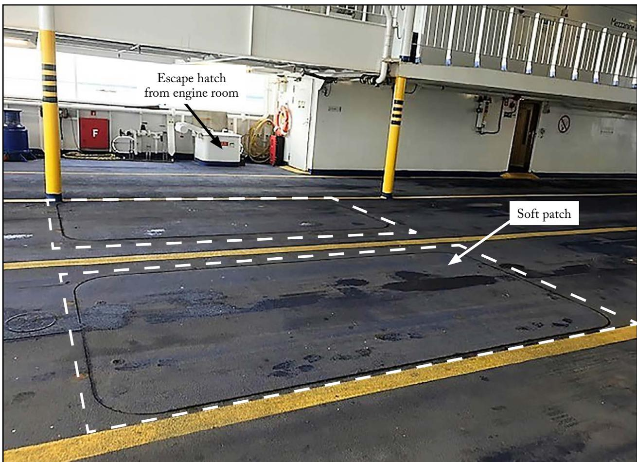
Figure 2: Soft patch and escape hatch
