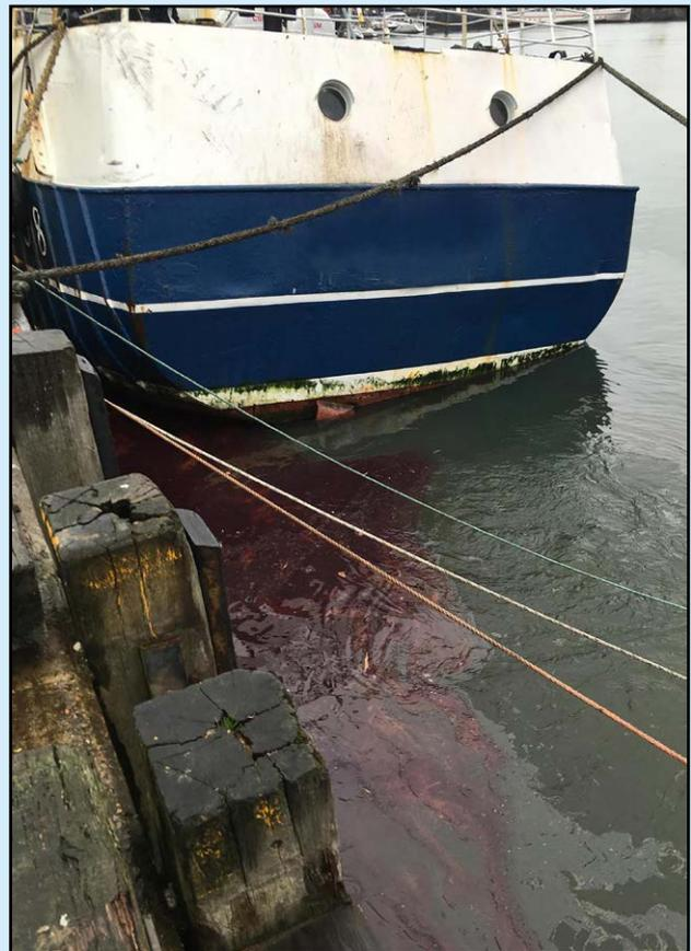
Figure: Pollution from the overflowing fuel tank
