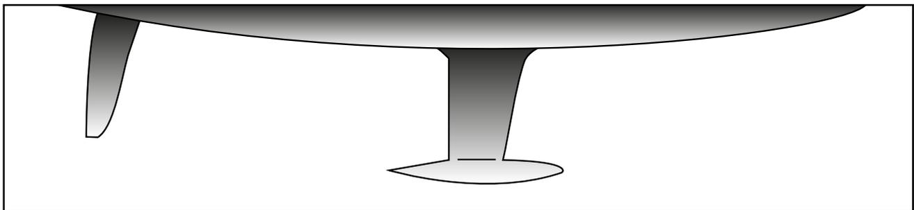
Figure: Modern keel and rudder arrangements are efficient but potentially vulnerable and should be professionally examined following a grounding
