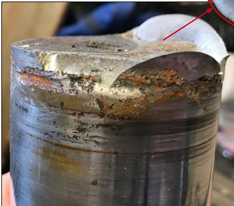
Figure 1: The failed rudder stock showing the effects of crevice corrosion
