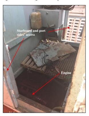
Figure 17: Starboard and port side engine-room access
