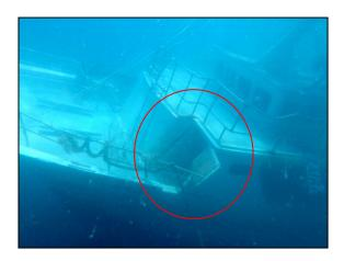
Figure 10: Door leading to the port side deck found in two pieces
