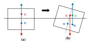
Figure 18: (a) the vessel in an upright position and (b) the vessel heeled to one side with  $B_1$  indicating the shift in the centre of buoyancy
