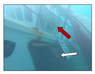
Figure 7: Port side of *Zaira*, red arrow showing the bridge hatch open, white arrow showing the port side bulwark hatch missing
