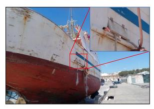
Figure 14: Magnified photo shows starboard side's freeing port. An identical freeing port was on the other side
