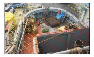
Figure 12: The poop deck of *Zaira*, showing a reconstruction of the sheltered deck (in yellow) and a reconstruction of the engine-room deckhead (in red)
