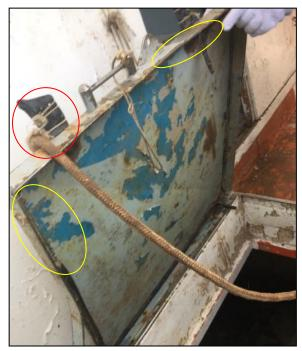
Figure 15: Hatch cover in way of fish hold, showing worn out rubber inserts (in yellow) and rubber strips around the securing points (in red)
