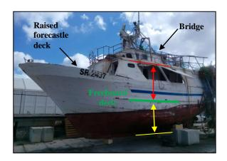
Figure 1: Zaira, from her port side. The moulded depth is indicated in yellow, and the bulwark is marked in red
