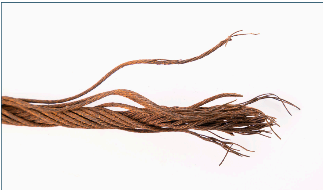
Figure 6: Parted wire from boat hook end Source: DMAIB
