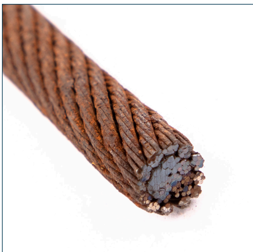
Figure 7: Sample wire 8m from the wire rope eye Source: DMAIB
