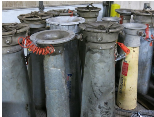
Types of air movers from IMT's shop used aboard the barge IB1940 on the morning of the explosion. (Photo taken after the explosion and after new bonding straps were attached to air movers.)
