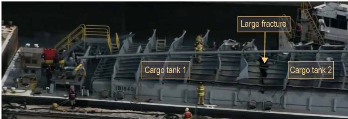
Aerial view of top side of the IB1940 after the explosion (Source: NBC News Chicago, annotated by NTSB)
