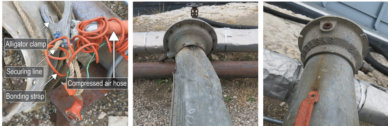
Air movers used aboard the IB1940 and removed after the explosion for inspection. Left: Alligator clip of bonding strap engaged in line of large blower. Center and Right: Small air mover with missing bonding strap.
