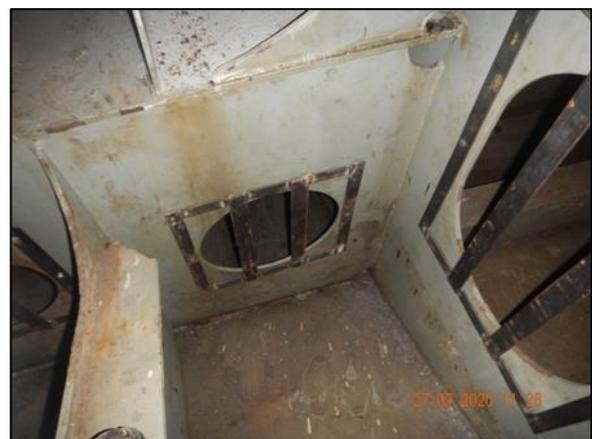
Figure 18: Lightening holes within the starboard bilge space blocked
