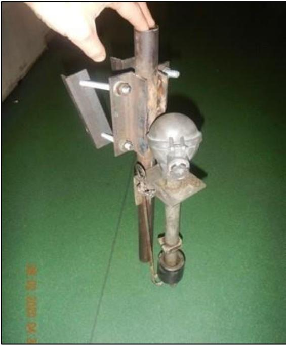
**Figure 3: Bilge alarm sensor (representative photograph)**
