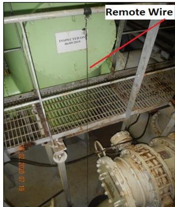
Figure 17: Wire to remotely test the starboard bilge alarm
