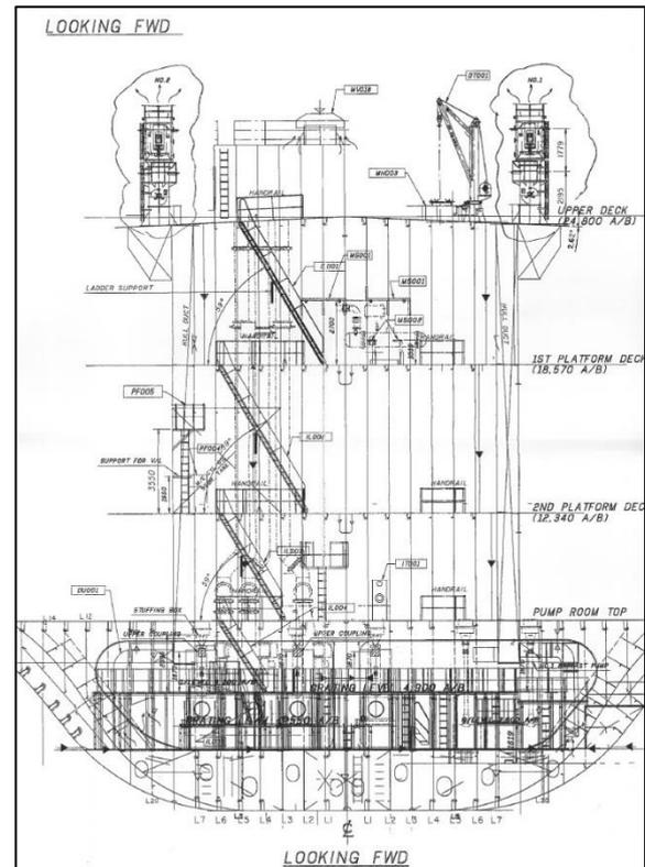
Figure 2: Pump Room Arrangement Plan
