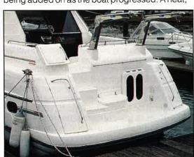
Sealine's latest and largest displays plenty of good design thinking, the foredeck area being a case in point. Here you find recesses for the anchor winch above and anchor below the stemhead platform, while fender stowages in the chain locker avoid the need for rail-mounted racks which would hinder visibility forward. Back aft, the locker theme has been extended to the bathing platform wings, with large stowages on both sides taking a passerelle, boarding ladder and more besides.
