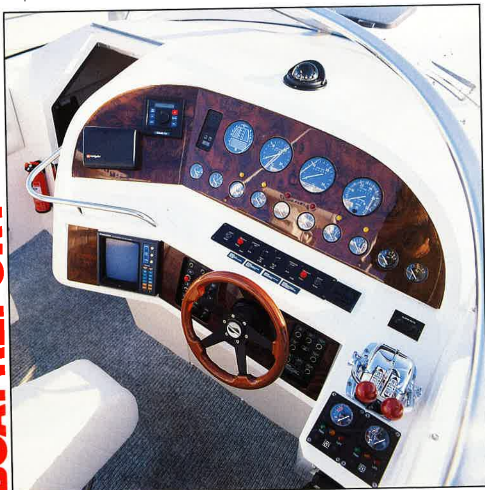
Left: now very much a Sunseeker trademark, the walnut dash is finished in epoxy to give a durable finish to a high-quality feature. And not only are the cosmetics of note but all items around the contoured helm fall easily to hand.
