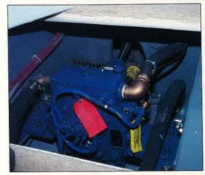
Our test boat was fitted with twin 230hp Volvo Penta KAMD42 diesels, located beneath the cockpit sole (right). driving through hydraulic vee-gearboxes nestling under the saloon (left).
