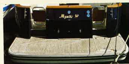
bathing platform This is not walled in by integral flanks, which makes boarding easy. Two teak-panelled transom gates lead forward into the cockpit.
