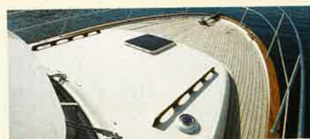
foredeck Very user-friendly, this has an electric windlass and single-chamber anchor locker.
