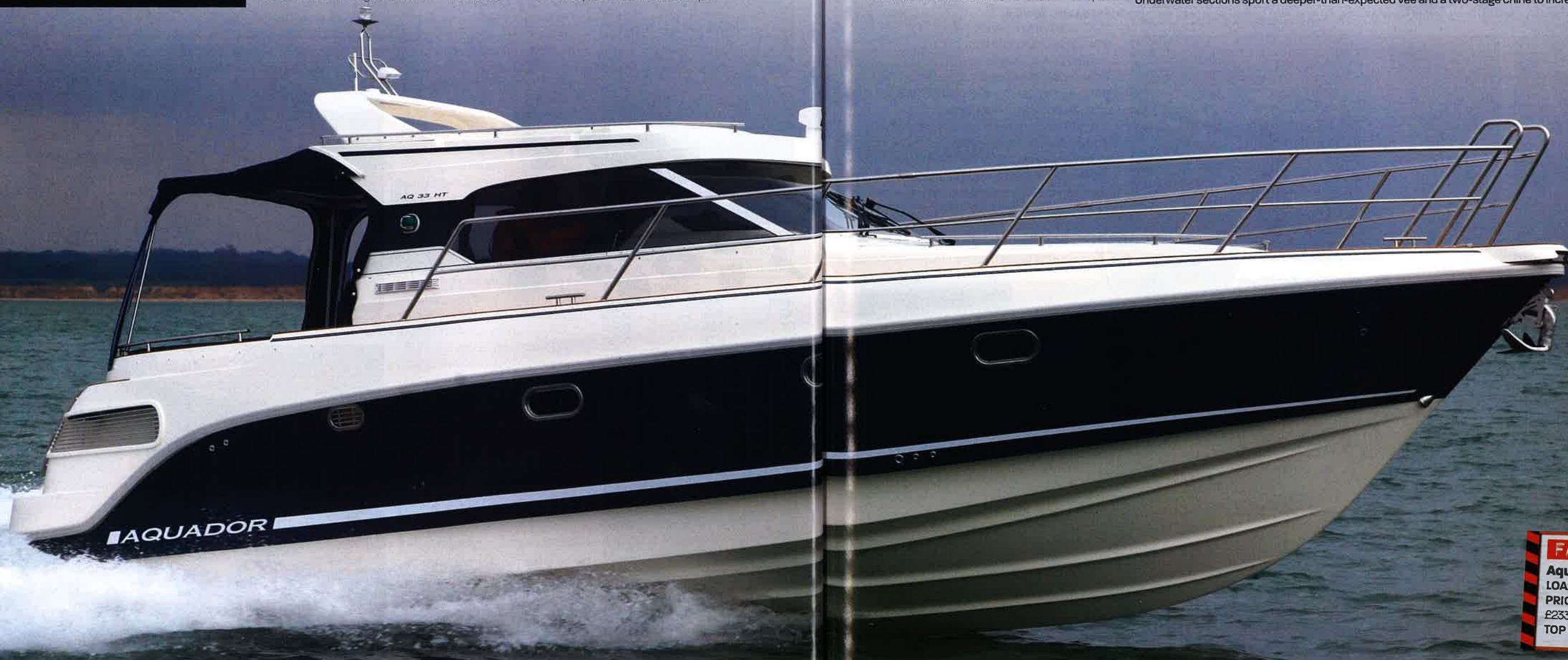
Underwater sections sport a deeper-than-expected vee and a two-stage chine to increase interior volume.
