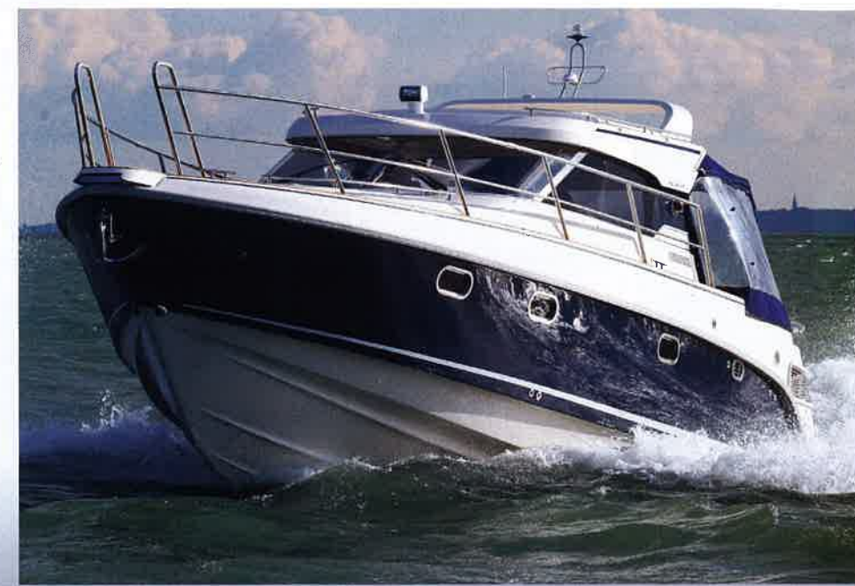
Underwater sections sport a deeper-than-expected vee and a two-stage chine to increase interior volume.
