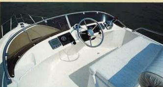
flybridge helm The layout of the upper helm spreads the controls out along a wide console. although everything is well within reach of the helmsman. Plenty of room is left for fitting extra navigational
