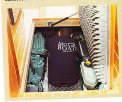
A separate service panel located above the port engine allows access to the fuel and oil filters, and the pre-filters and water filters are just about accessible at the rear of the compartment.
