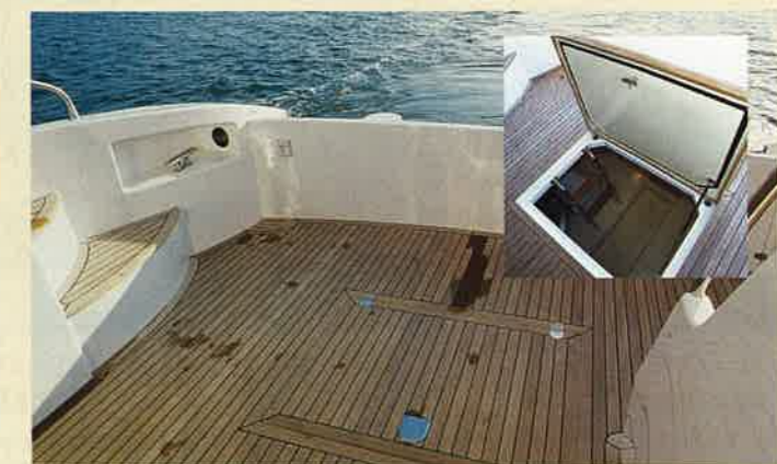
anchor locker This is thoughtfully fitted with a basket that will take several mid-size fenders.
