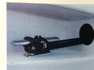
mooring Cleats on the quarters are hidden inboard, so that the warp has to be pushed through a pipe-type fairlead. This could do with more rounding off to prevent chafe.
