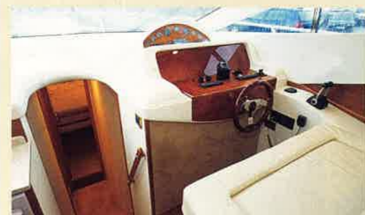
interior helm Smartly finished, the helm console is simply laid-out with instrumentation readily viewed. But the compass appears to have been surface-mounted as a bit of an afterthought.
