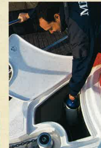
mooring Cleats on the quarters are hidden inboard, so that the warp has to be pushed through a pipe-type fairlead. This could do with more rounding off to prevent chafe.
