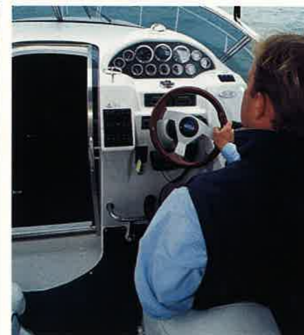
helm The dashboard gives a very good layout of instrumentation and switches, though room for adding more than one extra piece of electronic display is limited and there is no formal arrangement for chart display. A Simrad RD68 GMDSS VHF was included on our test boat as an optional extra.
