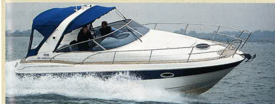
foredeck The opening in the pulpit allows for boarding at the bows if necessary.
