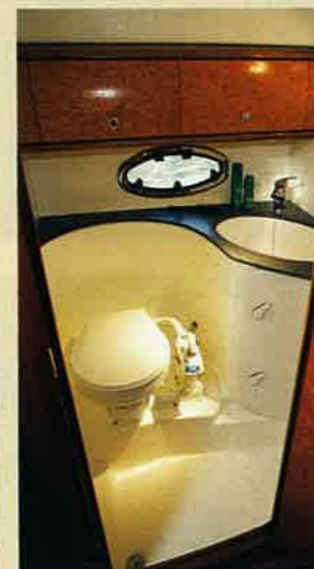
toilet/shower A stainless steel mixer tap on a wanderlead doubles as the showerhead, and a sea toilet with a manual flush comes as standard.
