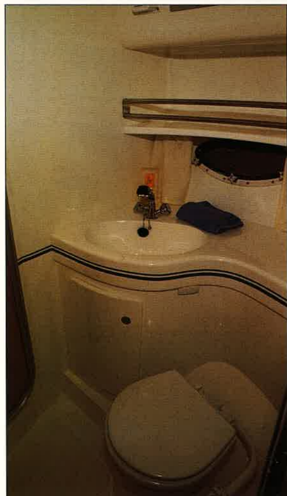
Above: the galley is three steps down from the saloon and to starboard, with natural light from a translucent panel overhead, a good selection of appliances but limited storage space. Left: the toilet/shower compartment is of sensible proportions and serves both sleeping cabins. The toilet discharges to a holding tank as standard, but a sea outlet is an option.
