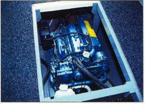
The compartment is lined in pegboard-style noise insulation, which gives reasonable results.
