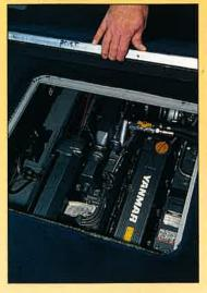
the primary fuel filters. On our test boat this required the aft companionway steps to be lifted clear, then a limbo through to their location on the aft bulkhead, although Broom have told us the installation will be modified to make servicing easier.
