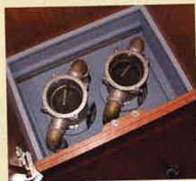
left A false bottom to the wardrobe in the aft cabin lifts out to reveal the clear-topped raw-water strainers.
