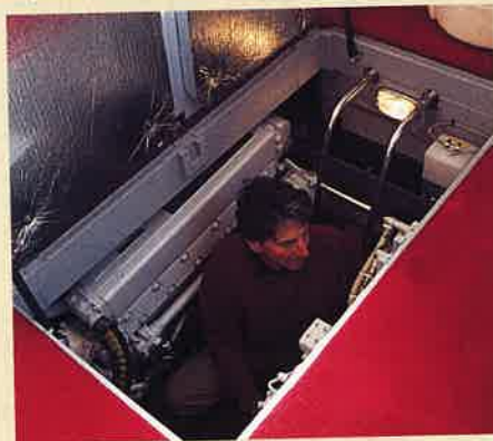
above A ladder and treadplate provide easy access down between the engines.
