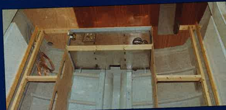
Many hours of careful, skilled work is required before a GRP craft can go into production. Key to the new boat's overall quality are the wooden plugs from which the moulds are taken. Seen under construction here at Brundall are (from the top) the plugs for the aft deck dodgers, hull and superstructure of the Ocean 34. Bottom: the cavernous engineroom of the first 34, before the sound-deadening fore and aft bulkheads were added (compare with the photograph on p75).
