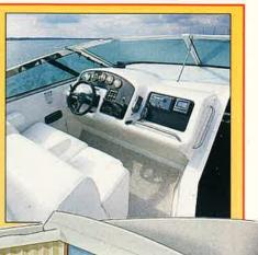
to hand. The throttles themselves, Twin Disc lectronic ones in the case of our test boat, are set inboard of the helm. while a wet-card compass is positioned nicely in the helmsman's line of sight.
