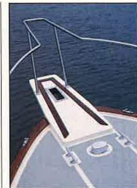
Above: the anchor platform belies the Chacewater's origins, but unlike on US-built craft, this extension to overall length is an optional extra. Above left: a cross-section through the hull, which features Airex foam sandwich build, constructed under the supervision of a composites specialist. Below: with room for two to sleep or four to sit, the interior is snug and practical for dayboating and overnighting.
