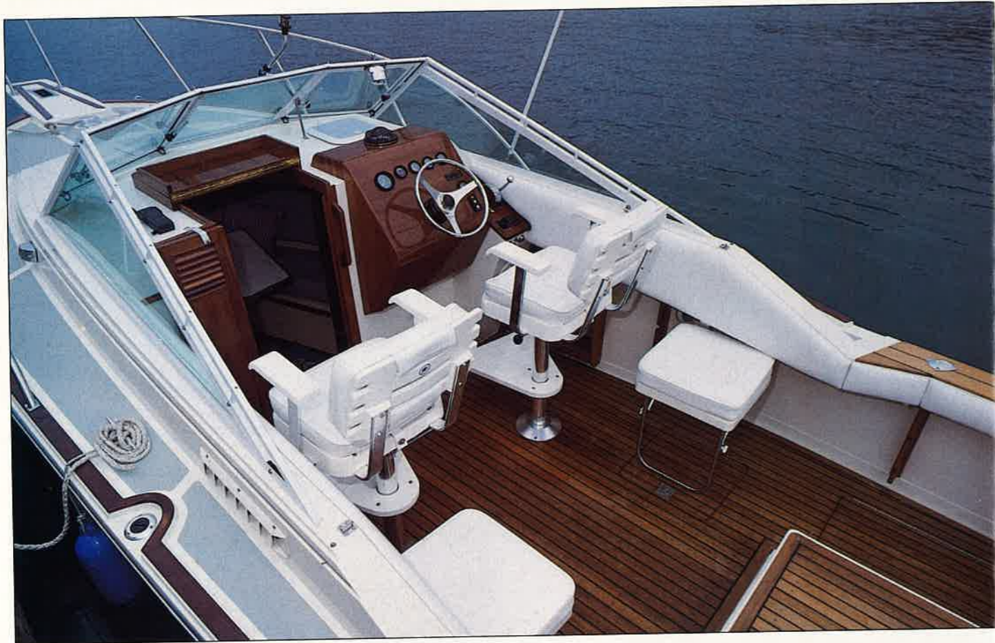
Above: acres of cockpit, together with jumpseats and rod-holders for the serious sportsfishermen amongst the crew. The highly polished teak console is an option; a GRP version with teak inlays is on offer for those seeking a more practical version. Below: the Volvo Penta KAD42 was a snug fit on our test boat, but Chacewater envisage giving more space to future installations.
