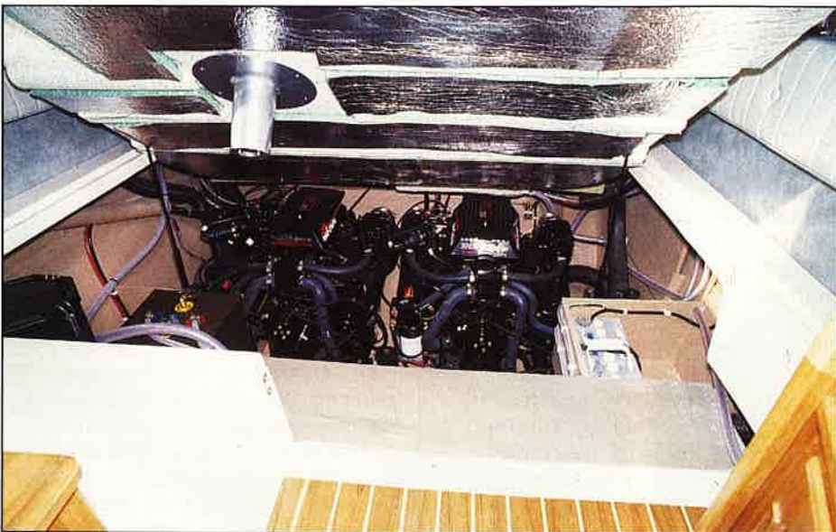
The whole cockpit sole lifts to reveal the engines.
