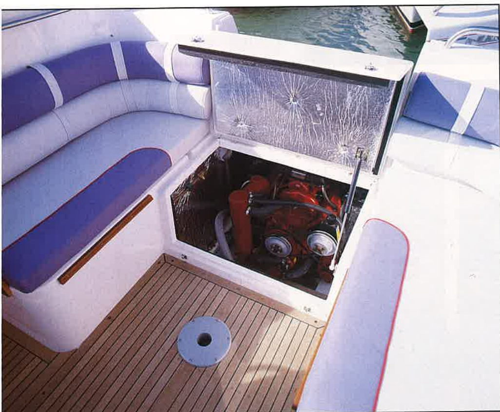
Good access to the 271hp Volvo through the aft seat/locker.
