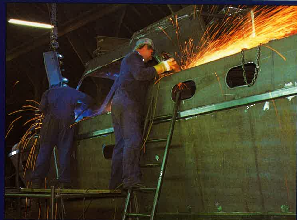
Bright sparks. Welding together a 40ft hull (above) takes just 10 days. The shell is then transported to a different yard to be grit-blasted and another for fitting-out (left).
