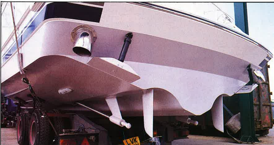
The business end of things, showing the propeller tunnels.
