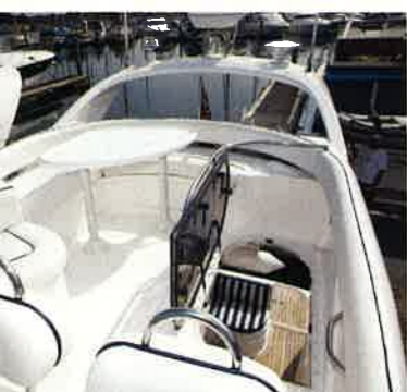
below The upper helm is well designed for three people, with each seat accessible independently.
