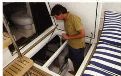
above A hatch with a gas strut gives access.
