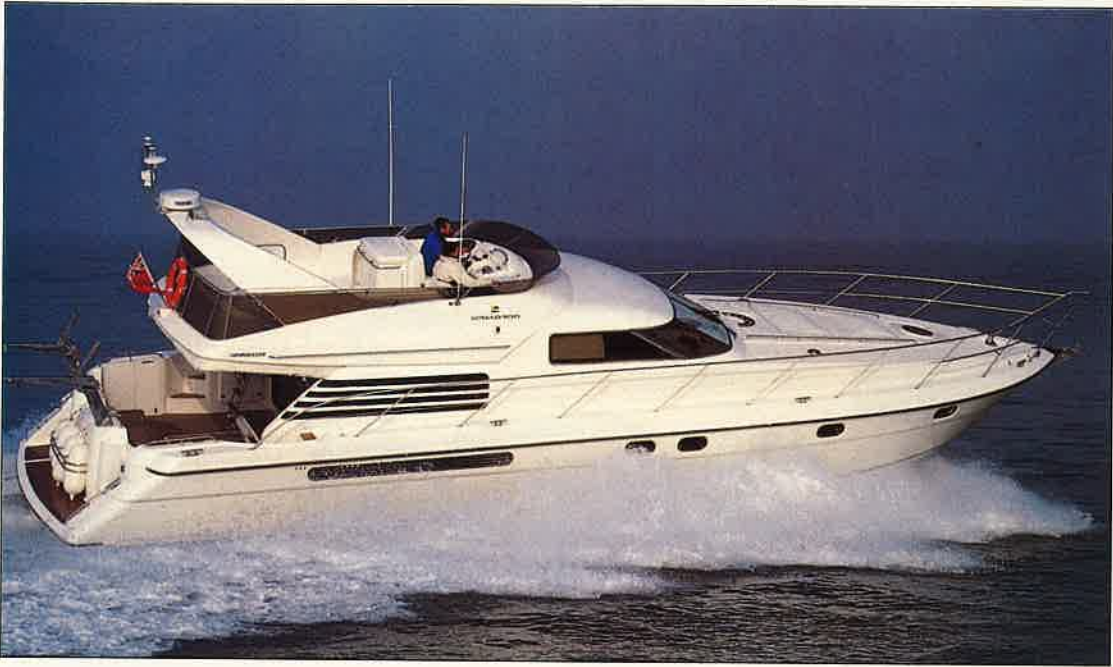
The 56's performance with twin 680hp MAN diesels was impressive, with acceleration up to 20 knots in less than 10 seconds and a top speed of more than 30 knots. Power steering means the Squadron can be thrown around like a sportsboat.
