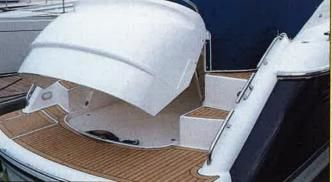
before you invade the cockpit. The garage will take an inflatable up to 9ft 4in (2.84m) complete with an attached outboard, which you simply haul up over the platform. The top of the hydraulically actuated lifting door (above), bordered by a handrail, doubles as a sunpad
