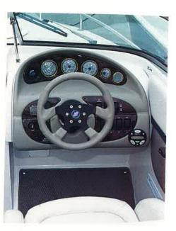
helm The dashboard, with its burl wood trim, displays all you need to know in an ergonomic format. The standard specification includes a compass, a digital depth-sounder and stereo controls. This leaves little room to fit extra navigation aids, but owners of this type of craft will probably only consider a handheld GPS anyway.
