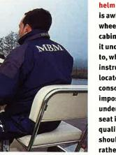
helm The helm position is awkward, as the wheel sits under the cabin overhang, making it uncomfortable to get to, while the engine instrument panel is located under the console, making it near impossible to view while underway. The raised seat is of a good size and quality, but we feel it should be removable rather than fixed.
