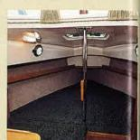
forward berth This double is separated from the dinette by a backrest that can be removed to enlarge the cushioned area. A stainless steel centre pole makes for a useful grab handle.
