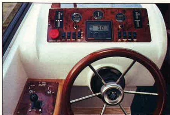
Above: the first Brimbelow electric-powered craft at home on the Norfolk Broads. Left: alongside the steering wheel is a single short joystick, which is used to control the boat's thrust, forward or astern, and to vary the speeds of the two motors.
