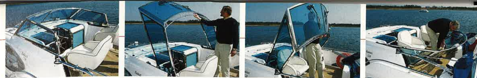
windscreen An innovative approach to squeezing under low bridges is this optional up-and-over arrangement, reducing air draught to around 8ft 3in.
