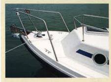
guardrails Inboard handrails lining the forward part of the superstructure make an easy transition to the pulpit rails.
