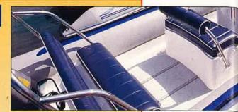
accessible locker under the bench. where the twin batteries are fitted, in addition to the good-sized locker in the base of the helm seat.
