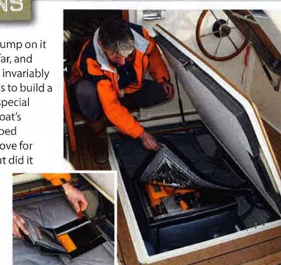
Interboat's neat idea of boxing in the engine reduces noise and all the service points are still accessible
