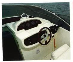
helm The console is on two levels, with walnut burr panels for the engine instrumentation and switches. A compass tops the dash, and there is plenty of space for fitting extra electronics. The wooden steering wheel makes a welcome change from the skinny steel wheels fitted by most of Jeanneau's competitors, but it has no tilt-adjustment.
