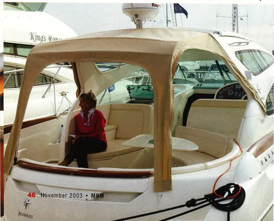
below An aluminium-framed canopy can enclose the cockpit. Access to the port side deck is easy.
