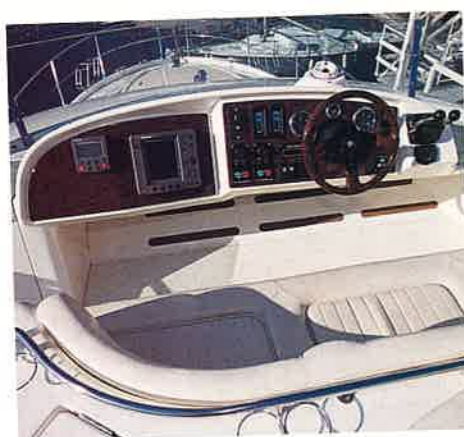
exterior helm Seating three, the flybridge driving position is tucked behind a high console which gives a good degree of protection. It has a good arrangement of instrumentation and controls, and also manages to incorporate a couple of handy 'bits' trays and a small locker.
