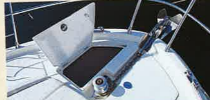
foredeck Sensibly, the locker is split between one compartment for the anchor chain and another for warps.
