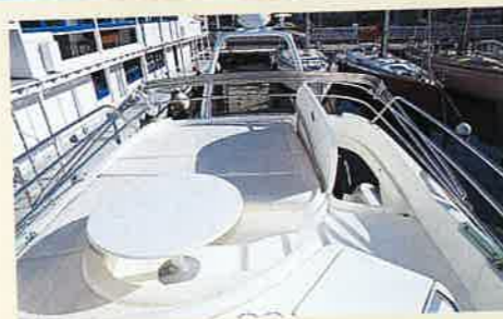
flybridge The coamings and seating are quite low, but are topped off with guardrails.
