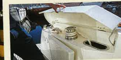
deckware Stern cleats and their associated rope bins are tucked beneath hinged lids, in this case with the optional docking winch, while the adjacent coamings are topped with chunky wood handrails.
