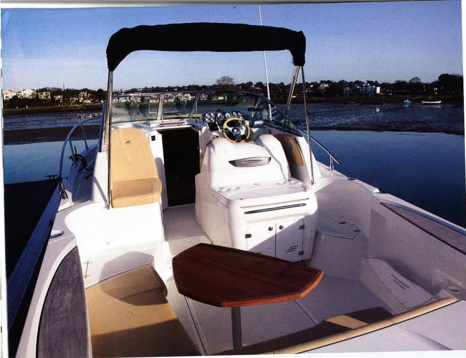
Smart and well laid out but flat cushion bases and no grab-rails makes holding on tricky in this 40-knot boat
