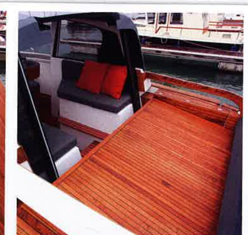
Up goes the decking, then the bulkhead slides down at the touch of a button – like an upside down garage door – and then the decking covers it up
