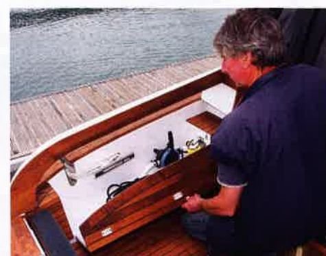
The cockpit coaming doubles as seating and storage
