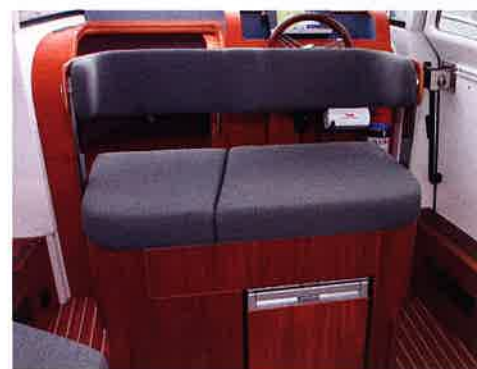
The helm seat's backrest flips over to face the rest of the seating; remove the cushion to reveal the hob
