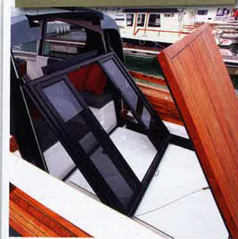
Up goes the decking, then the bulkhead slides down at the touch of a button – like an upside down garage door – and then the decking covers it up
