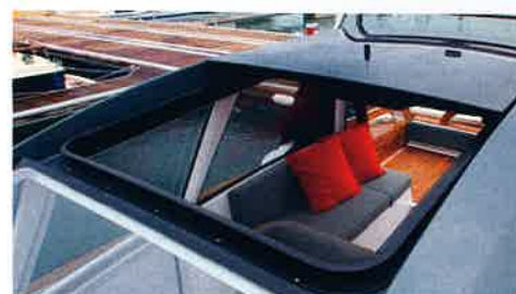
The sunroof opens in two sections that tuck underneath each other
