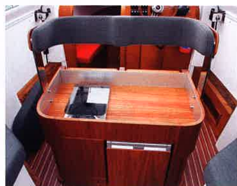
The helm seat's backrest flips over to face the rest of the seating; remove the cushion to reveal the hob
